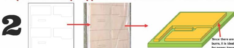
Sanko-Giken offers innovated heavy copper PCB using Fine Blanking Molding process to make up to 5mm thick power traces.
